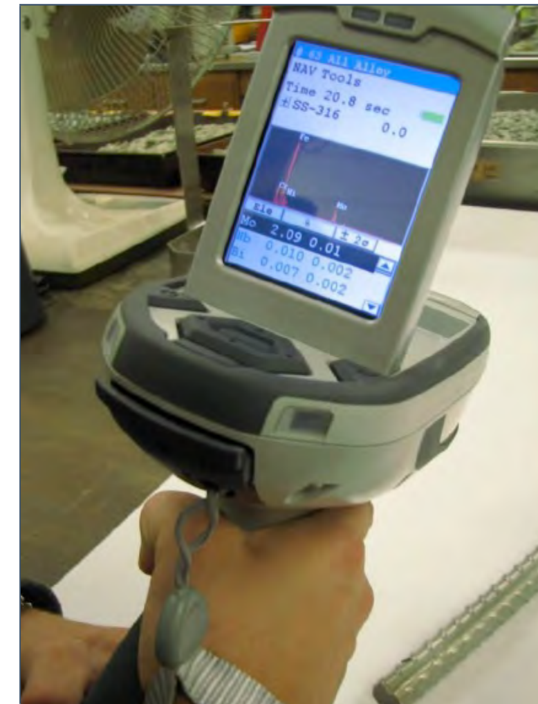
Figure 32. Hand-held X-ray fluorescence device as used by Virginia DOT
