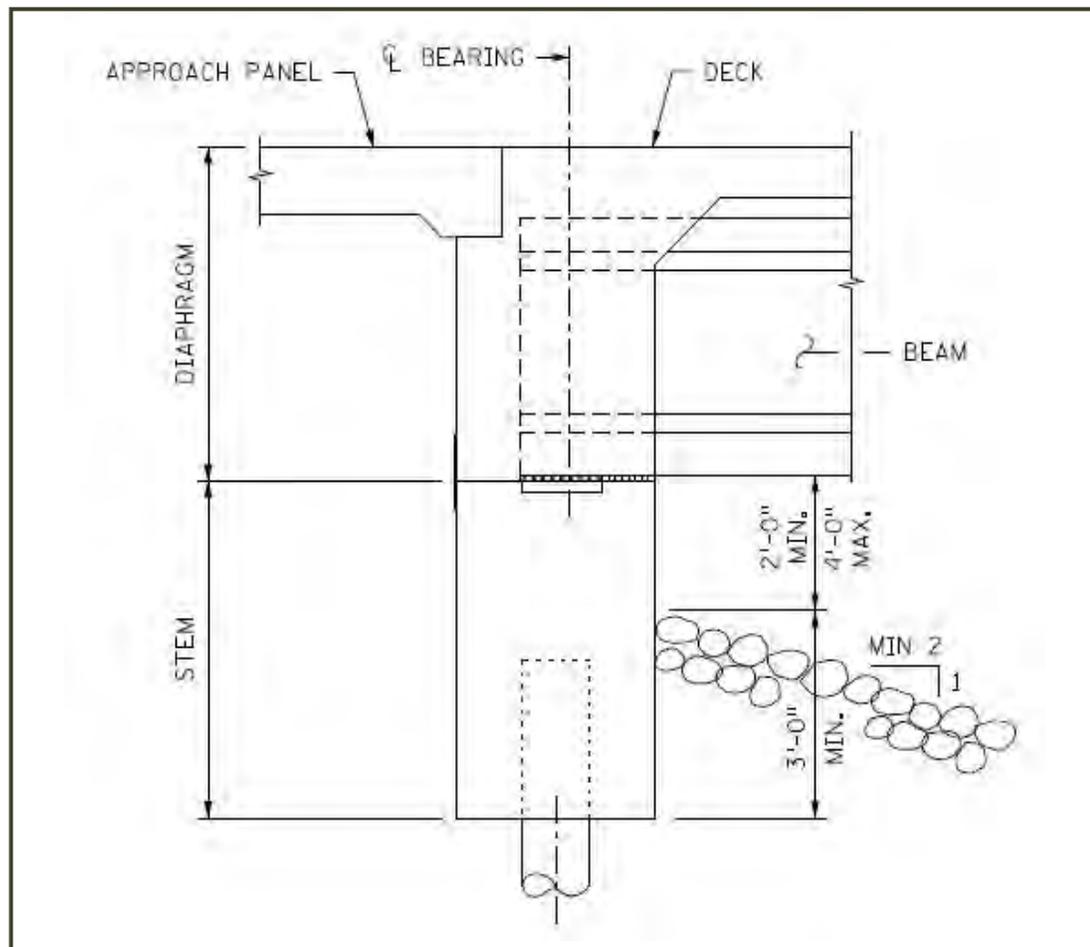
Figure 33 Integral Abutment Detail (courtesy MnDOT)
