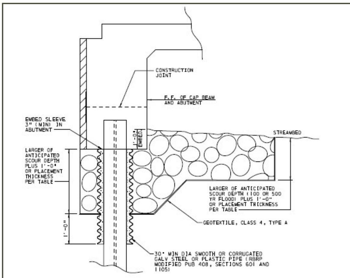
*Figure 52 PennDOT Alternate Scour Protection Detail*
