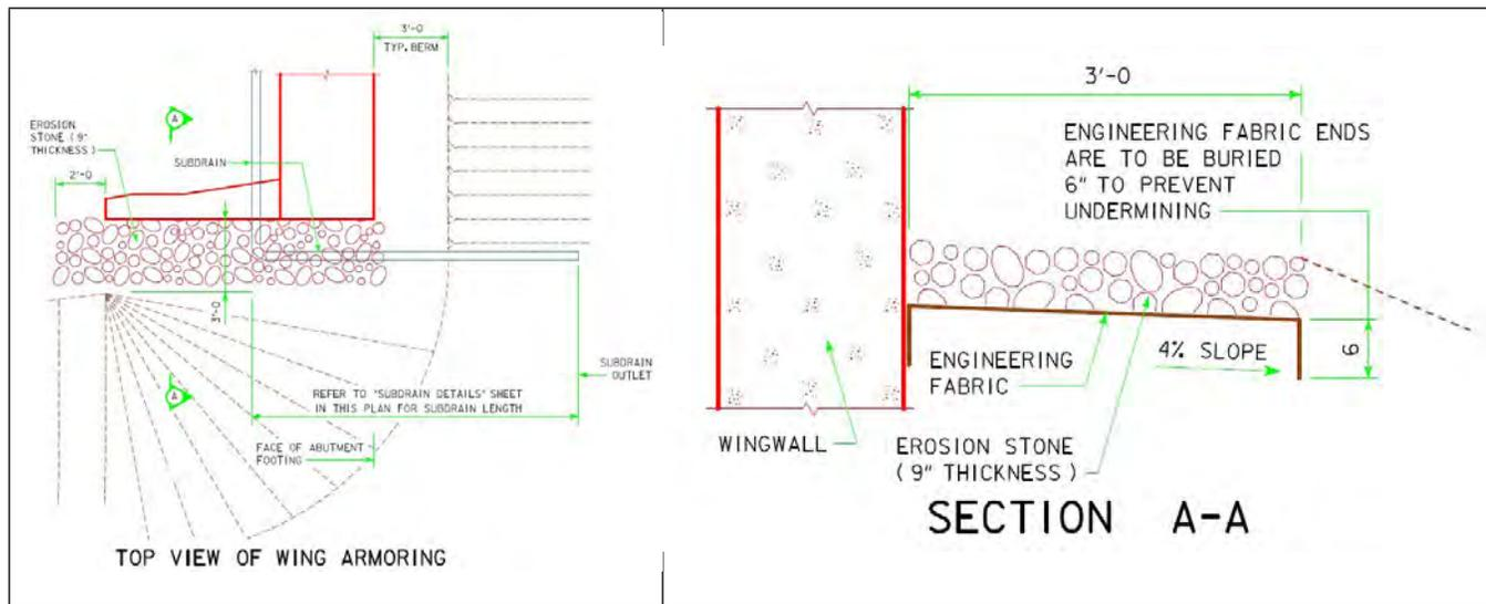
**Figure 48 Iowa DOT Wing Armoring**
