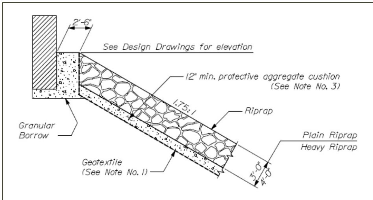
**Figure 49 MaineDOT Riprap Slope Integral Abutment**
