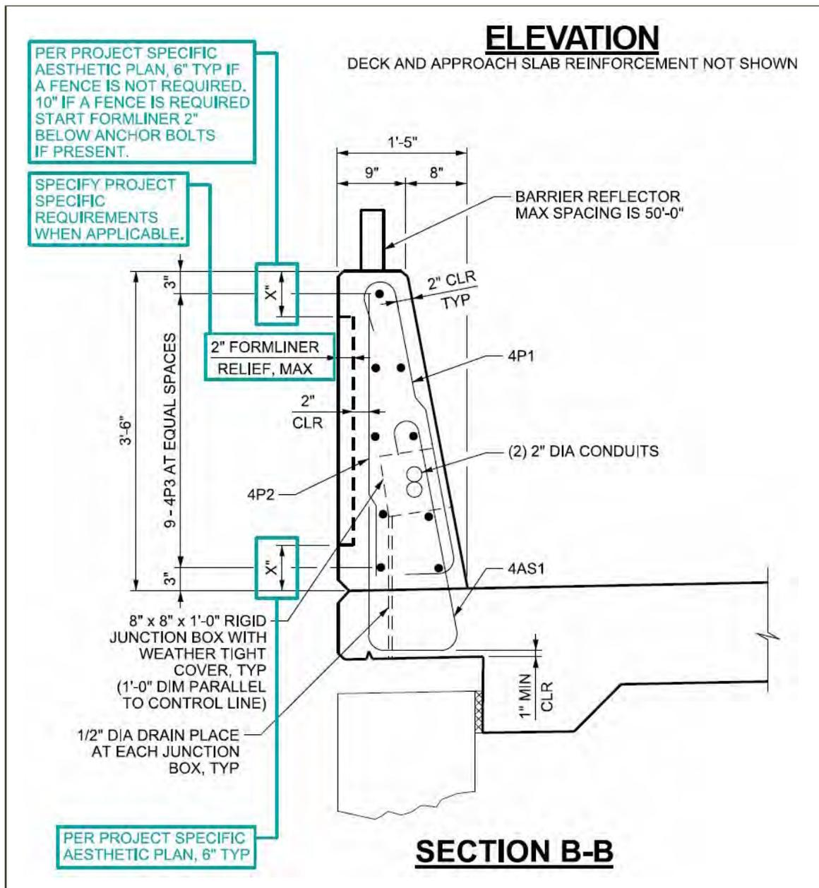
Figure 88 UDOT Barrier Rail
