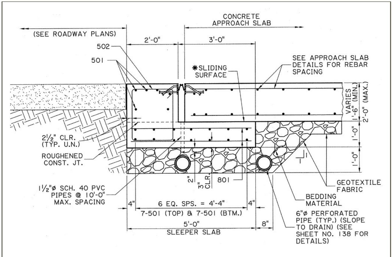
Figure 76 LaDOTD Slab to Pavement Connection
