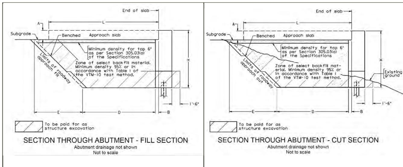
**Figure 98 VDOT Select Backfill**
