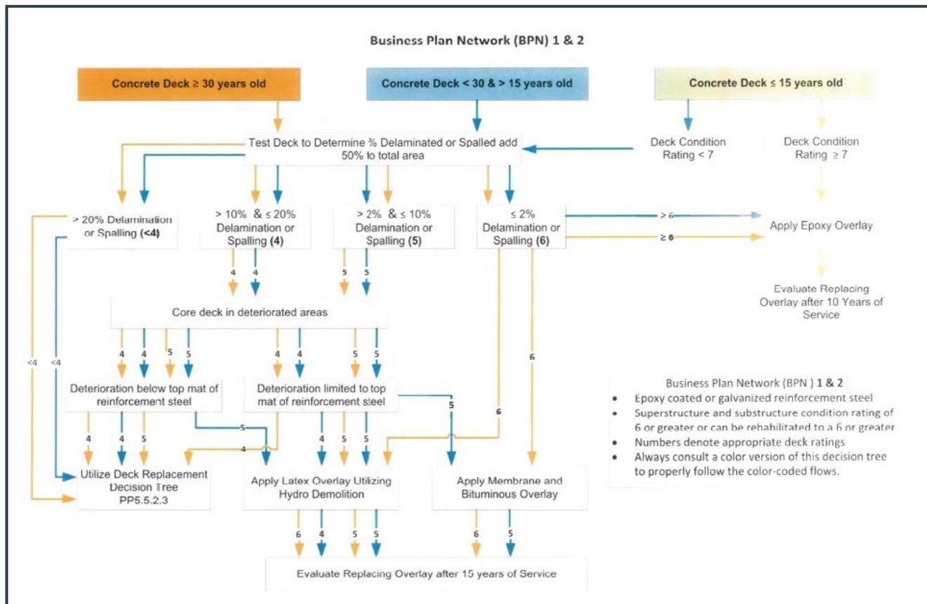
Figure 2-1 Concrete deck overlay decision tree for business plan network 1 and 2 (Pennsylvania DOT)
