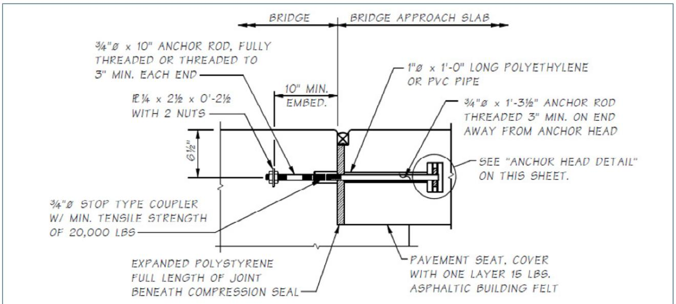
Figure 2.4-6. Approach slab connection detail.
