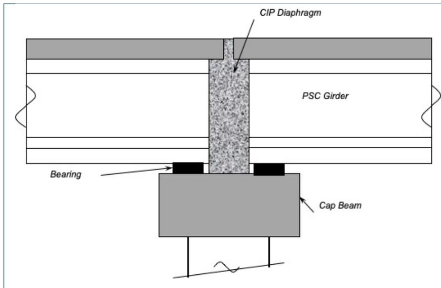
**Figure 2.4-1. Girders connected only to each other.**
