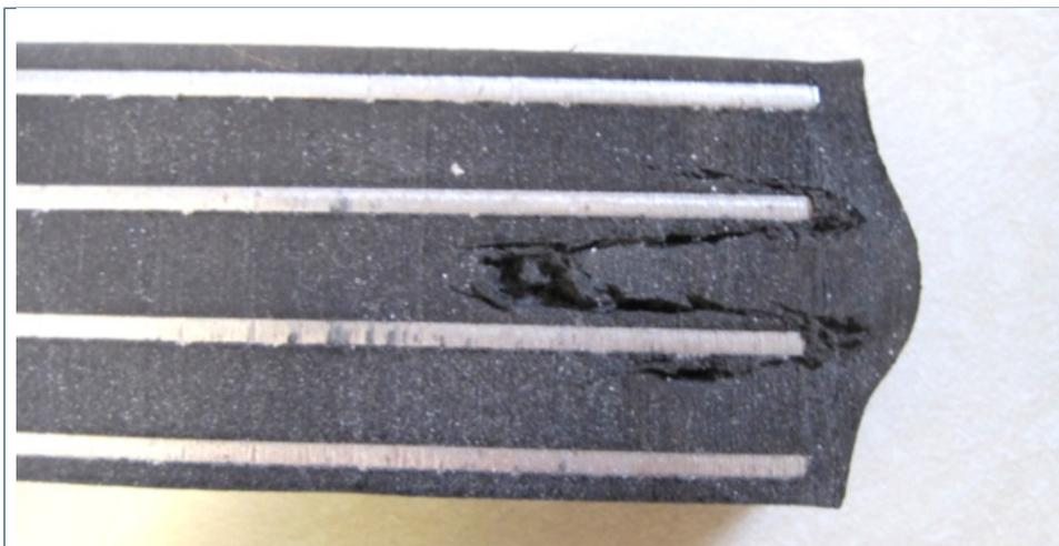
*Figure 2.3-40. Damage (in Test) to SREB due to severe overloading*
