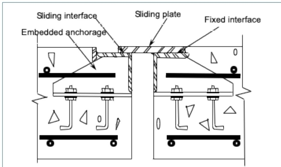
*Figure 2.4-34. Steel Sliding Joint*
