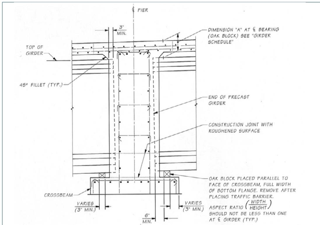
**Figure 2.4-2. Pier connection: girders and cap beam connected. (WSDOT)**
