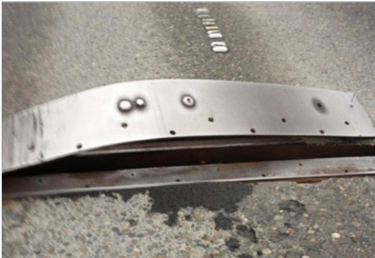
*Figure 2.4-35. Sliding plate failure (WA)*
