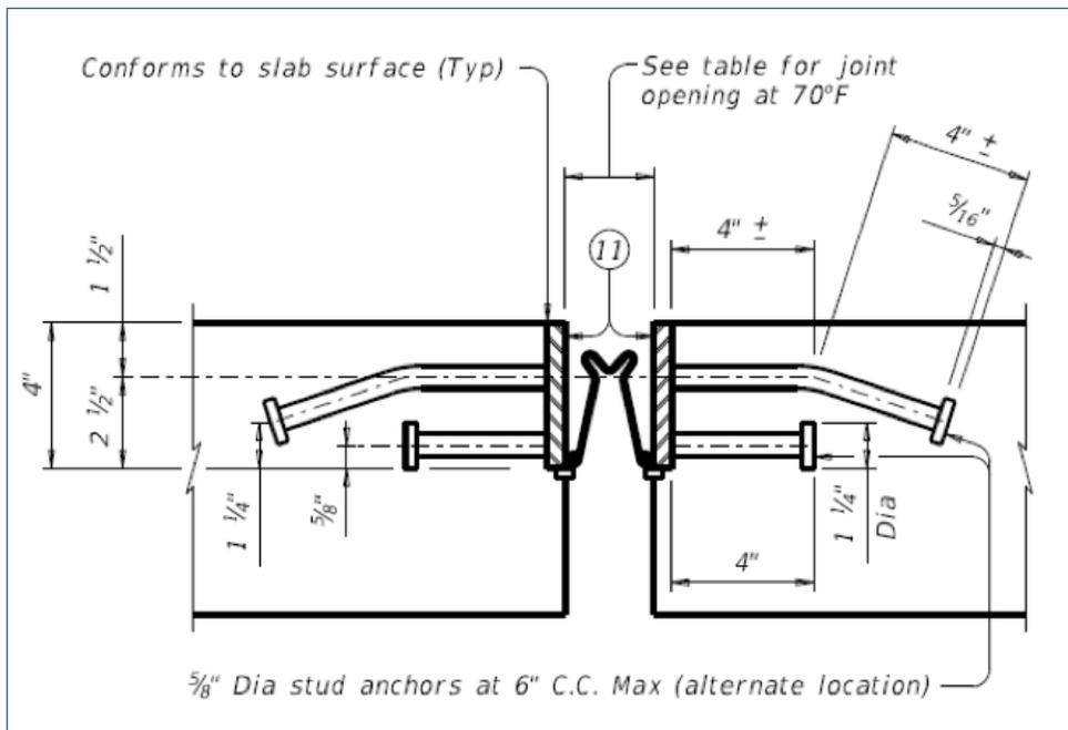
Figure 2.4-28. Gland-based seal: adhesive bonded strip seal, with armor
