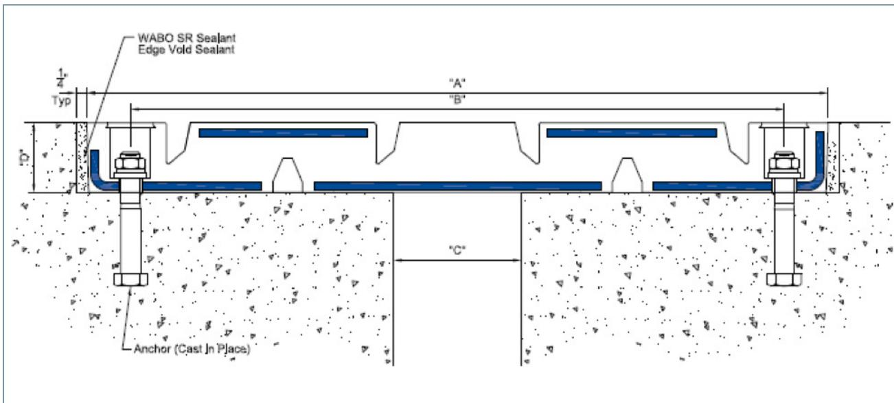
Figure 2.4-32. Bolted-on elastomeric panel
