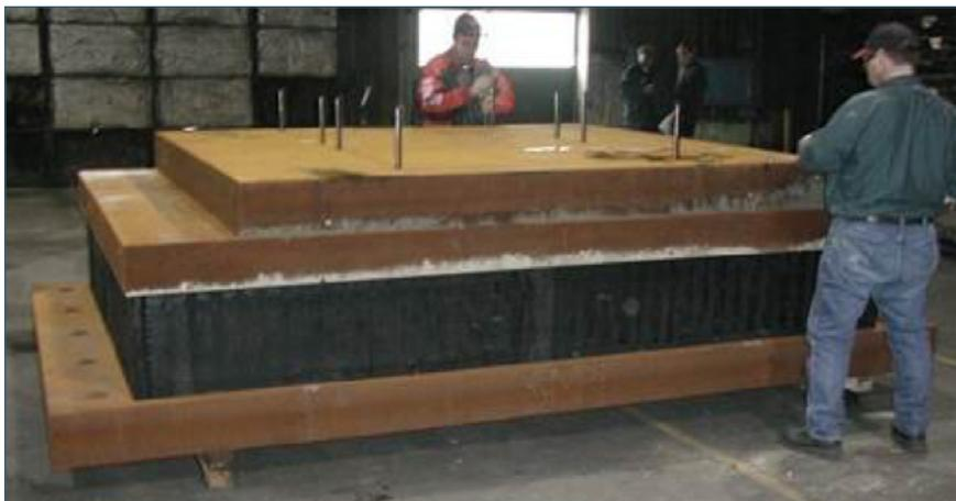
*Figure 2.3-3. Large elastomeric bearing*
