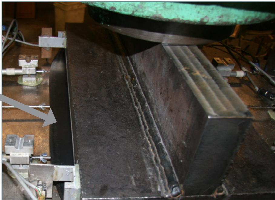
*Figure 2.3-19. Plain elastomeric pad squeezing out during test*
