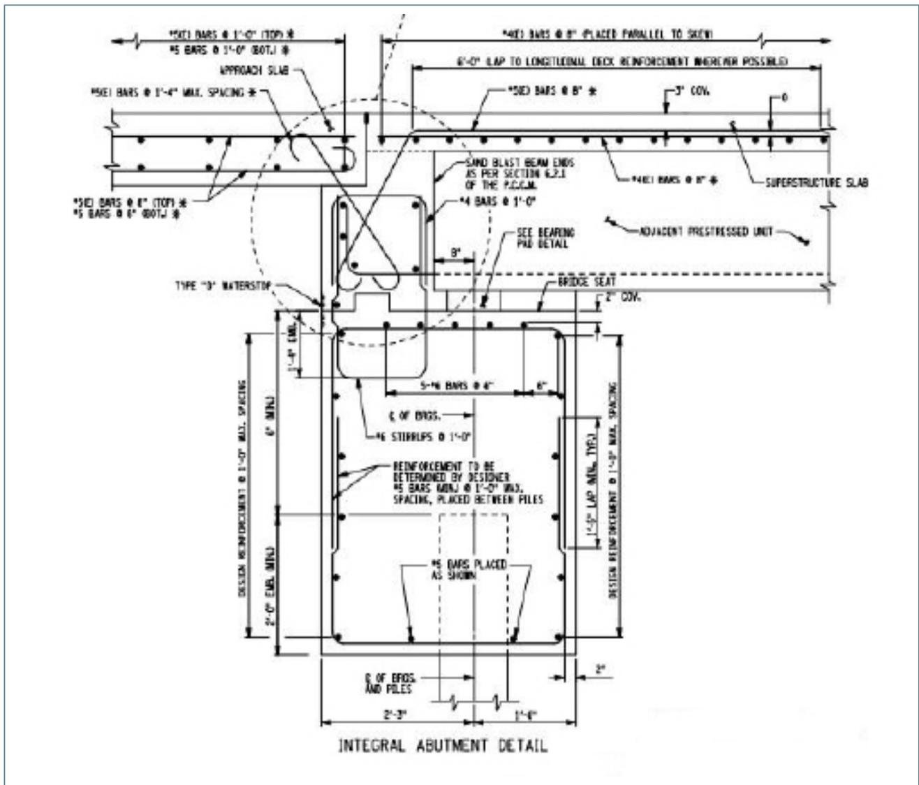
**Figure 2.4-5. Integral abutment**
