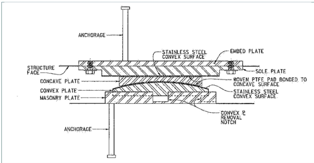
Figure 2.3-37. Bolted attachment detail for minimal lifting
