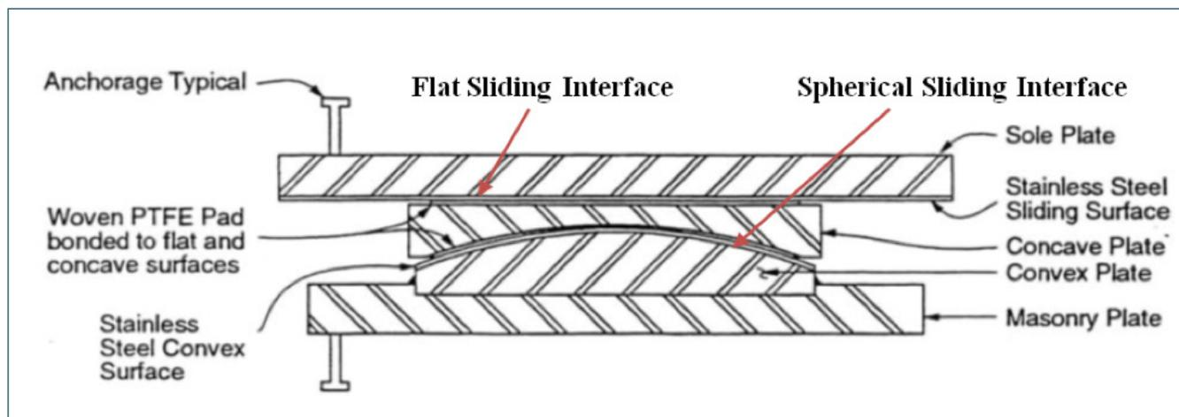
*Figure 2.3-23. Spherical Bearing (CA)*
