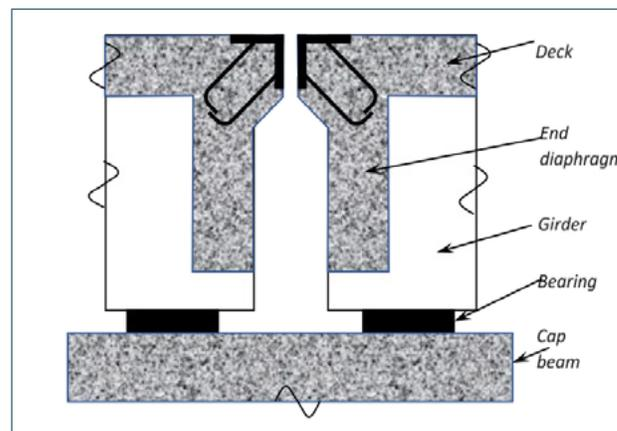
Figure 2.4-18. Open Joint
