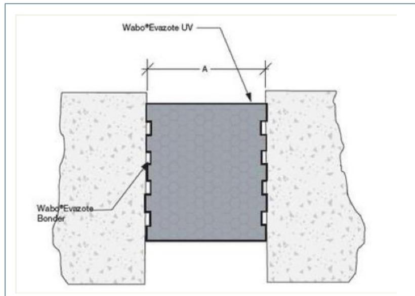
**Figure 2.4-23. Pre-formed compressible closed cell foam seal. [WA]**
