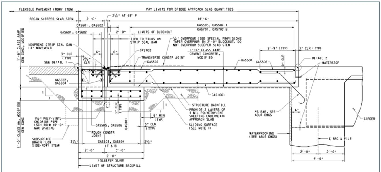
Figure 2.4-7. Sleeper slab detail
