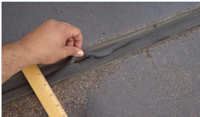
**Figure 2.4-24. Failure of silicone-coated foam seal (NY)**
