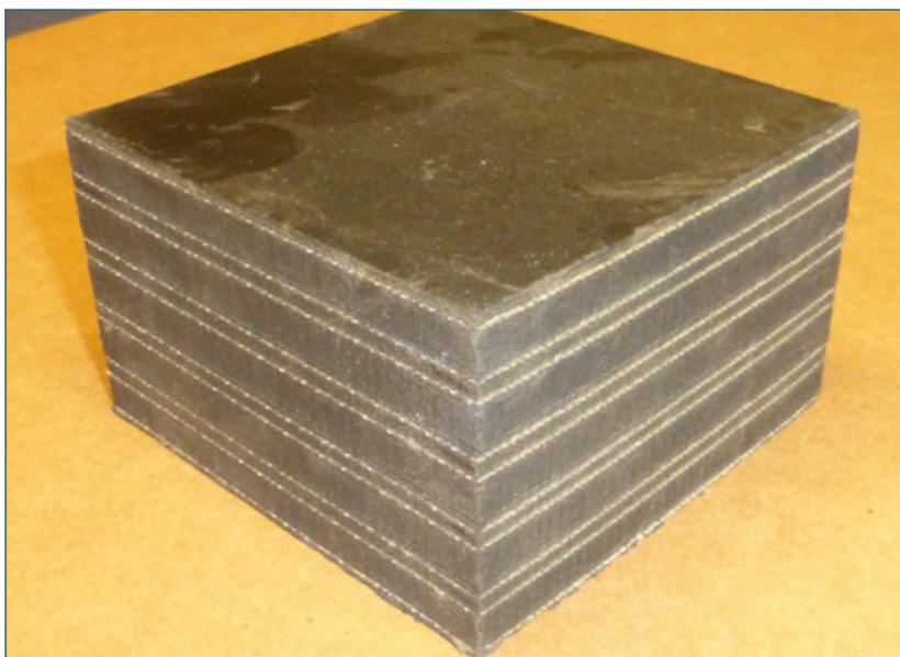
*Figure 2.3-17. Fiberglass-reinforced bearing pad (CA)*
