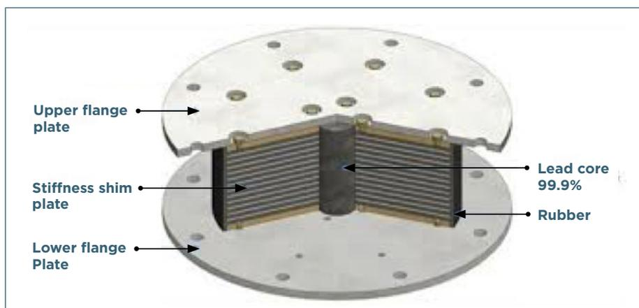
**Figure 2.3-25. Lead Rubber Isolation Bearing (DIS)**
