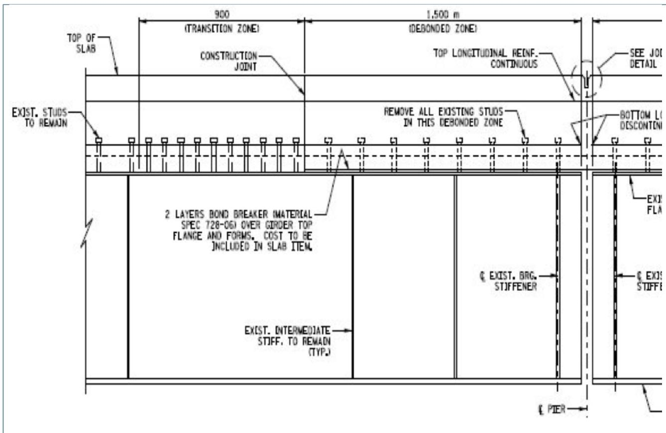
Figure 2.4-4. Shear studs removed from girder end (VA)
