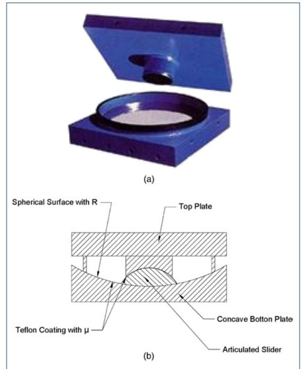
**Figure 2.3-26. Friction Pendulum Isolation Bearing**
