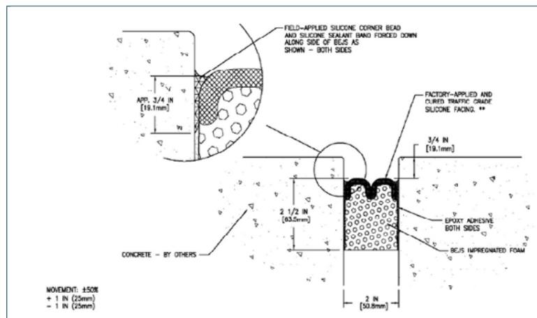
**Figure 2.4-22. Preformed (Impregnated open cell) foam seal with silicone facing**
