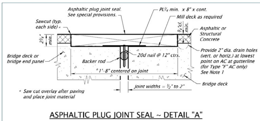
Figure 2.4-19. Asphaltic Plug Joint
