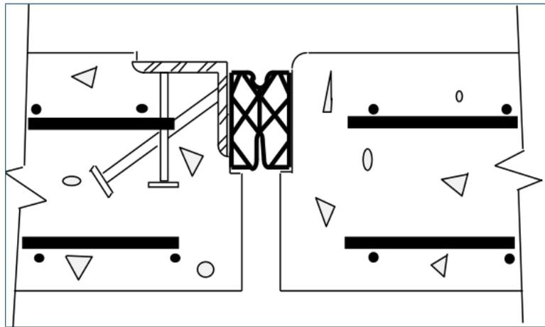
**Figure 2.4-21. Compression seal, with armor (left), without armor (right). [WA]**
