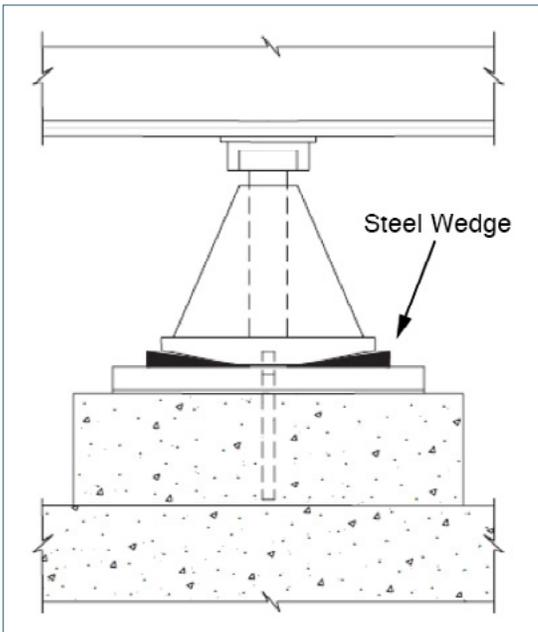
**Figure 2.3-4 Steel wedge detail for rocker bearing (from FHWA).**
