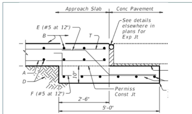
Figure 2.4-8. Alternative sleeper slab detail
