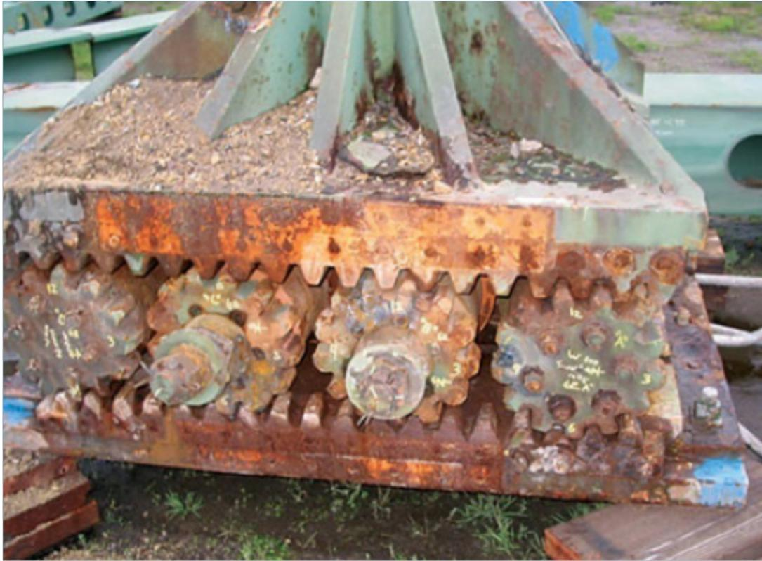
*Figure 2.3-38. Roller nest – serious corrosion*
