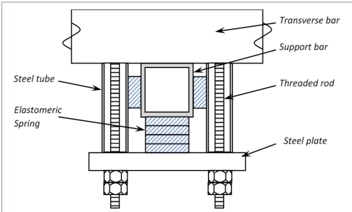
Figure 2.4-16. Bolted fix for failed welded stirrup in modular joint (OR)
