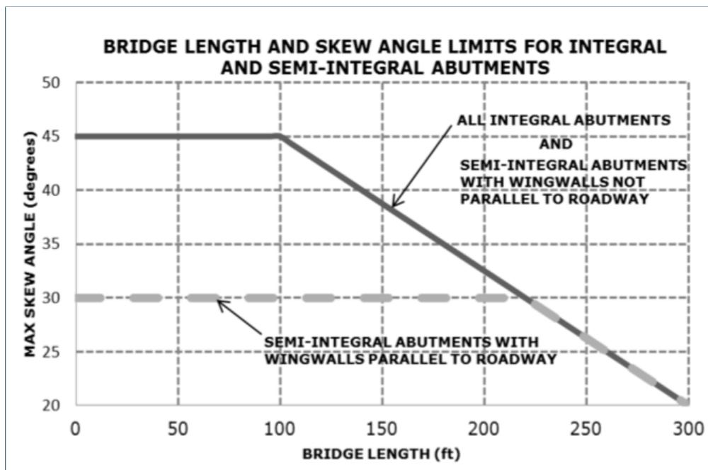
Figure 2.4-14. Skew and span limits on the use of integral abutments (MN)
