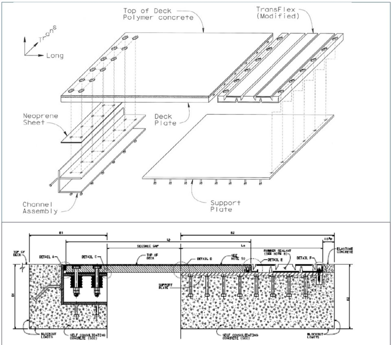
Figure 2.4-36. California Plate Joint Seal Assembly (Type II). Isometric and Section
