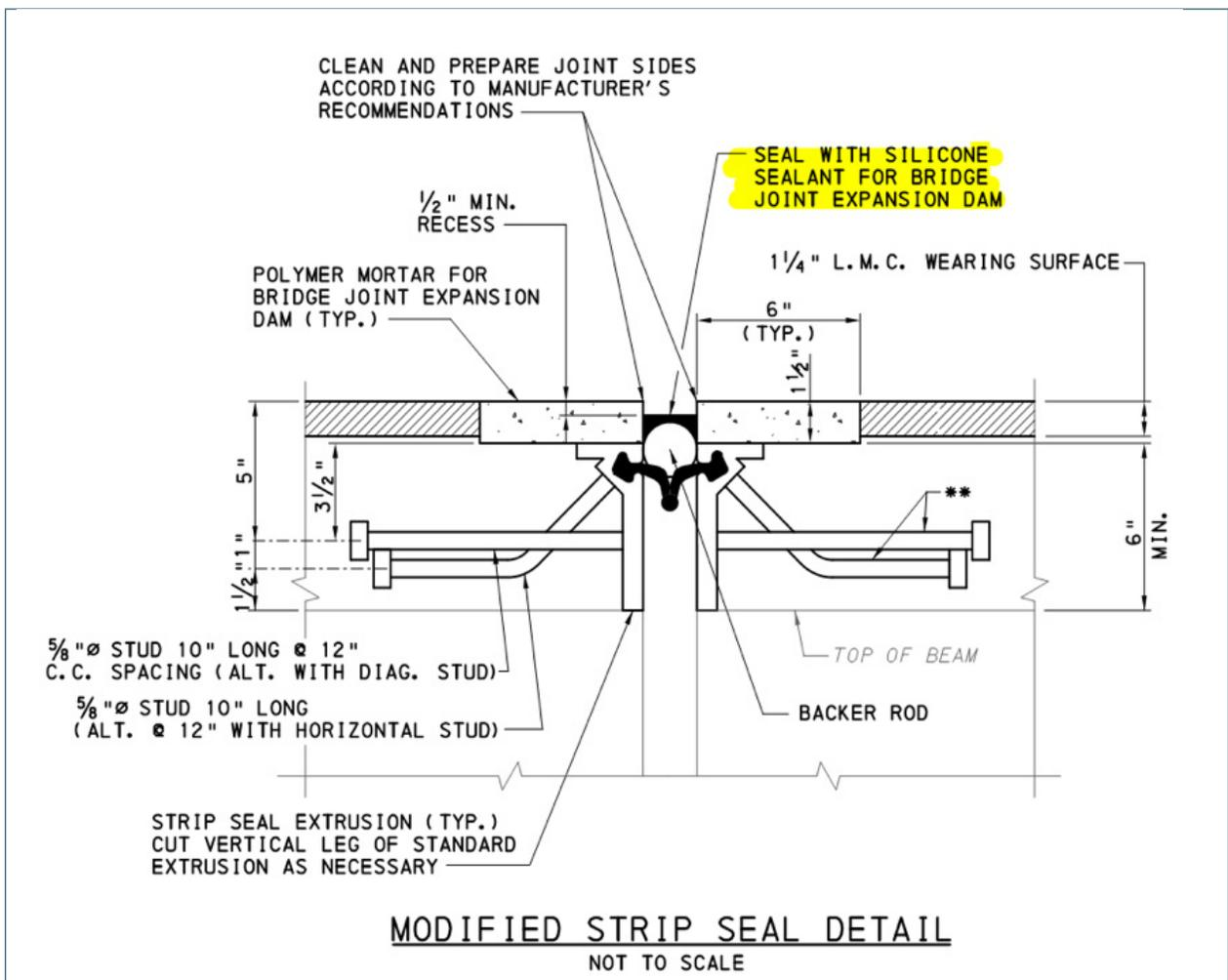
Figure 2.4-48. Strip seal modification to accommodate overlay
