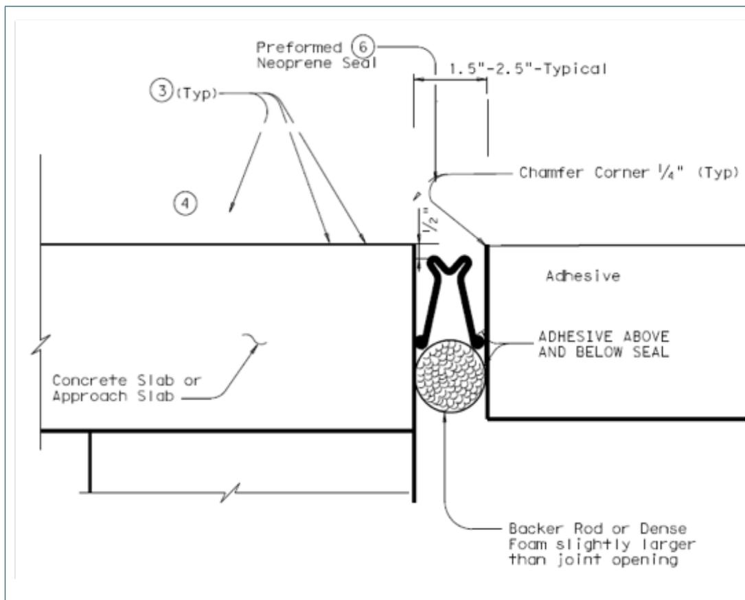
**Figure 2.4-29. Gland-based seal: adhesive bonded strip seal, without armor**
