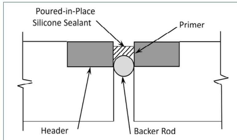
*Figure 2.4-20. Poured Seal (with backing rod)*
