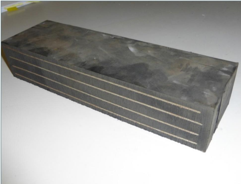
*Figure 2.3-13. Steel reinforced elastomeric bearing pad (shown cut open). (CA)*
