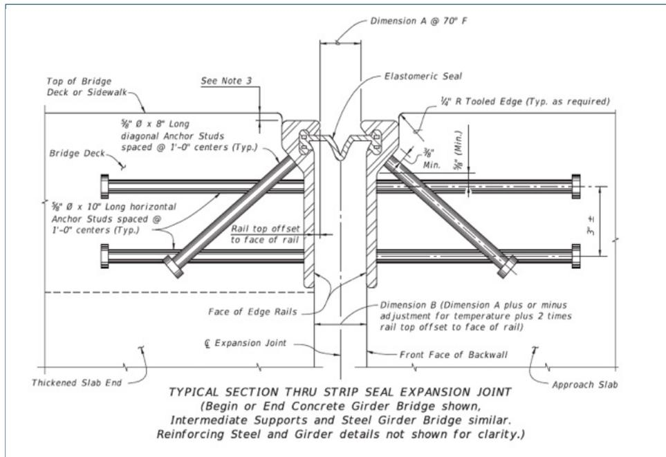
Figure 2.4-27. Gland-based seal: mechanically bonded strip seal (WABO)
