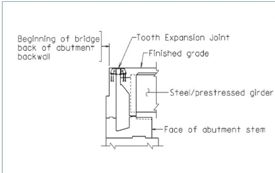
**Figure 2.4-12. Virginia abutment: cross-section**
