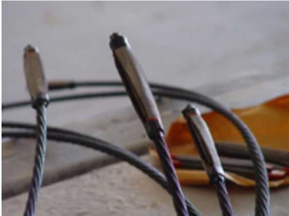
Figure 2-25 CFRP cable and end grip used for P/S
