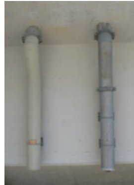
Figure 3-39 FRP pipes being evaluated against steel
