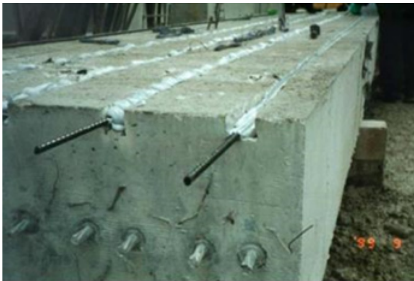
Figure 2-24 FRP reinforcing bars encased in adhesive as part of a NSM concrete strengthening system. (Note that this is in a laboratory setting.)
