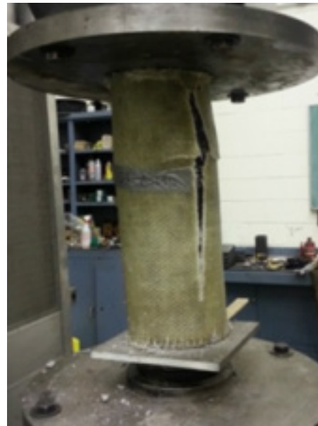
Figure 2-48 A timber pile similar to the one in Figure 2-47 failed at a much higher load due to confinement provided by the FRP wrap
