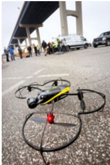
Figure 3-55 Lightweight carbon is used for this inspection drone, an emerging technology.
