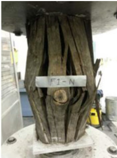
Figure 2-47 A timber pile that has failed due to buckling of the natural fibers under compressive loads
