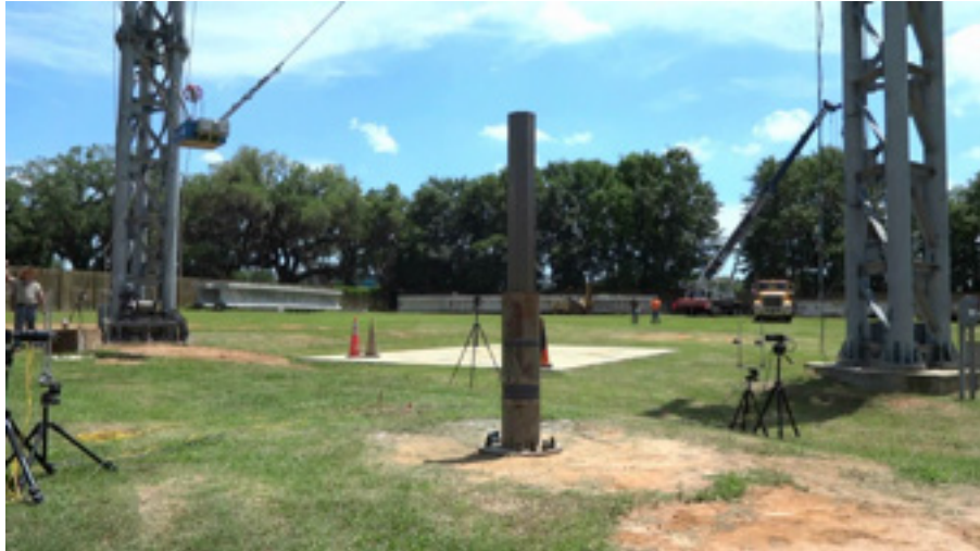
Figure 3-54 FDOT testing a breakaway base for an FRP pole
