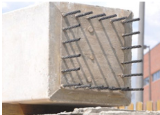
Figure 3-5 Concrete pile P/S with CFRP
