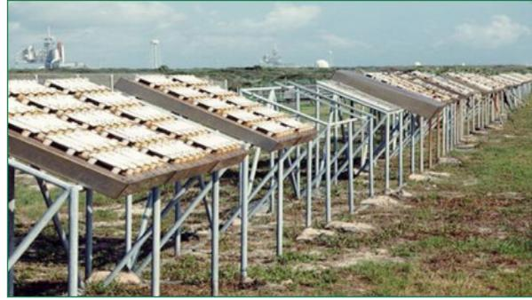
**Figure E 2** *Test panels exposed to weather at the Kennedy Space Center test site*
