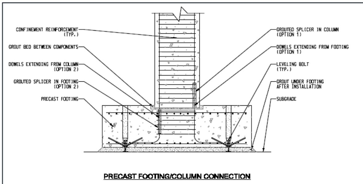
Figure 2.9 Precast footing to precast footing connection
