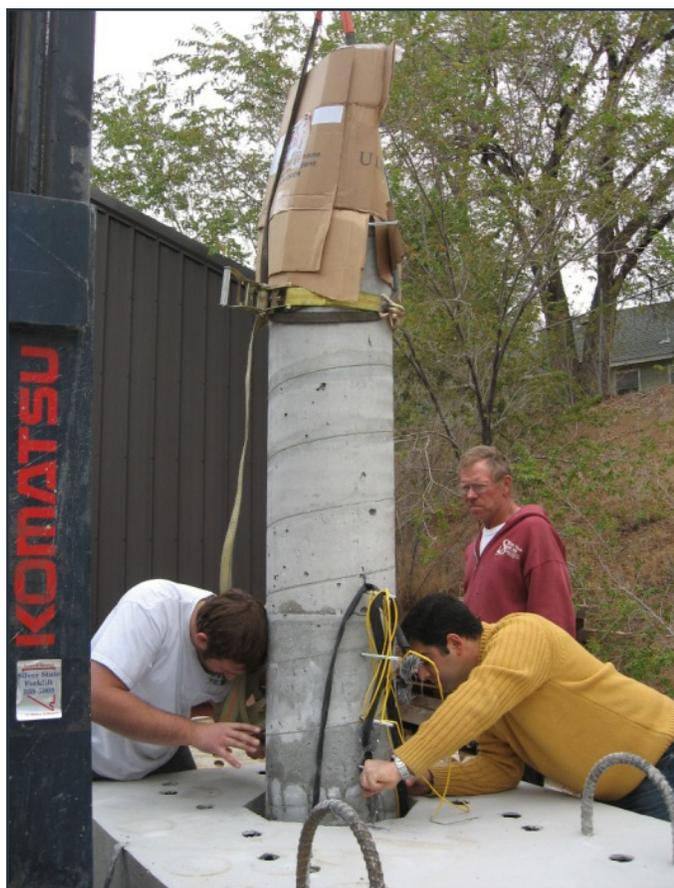
Figure 2.16 Precast column to precast footing connection in a UNR study
