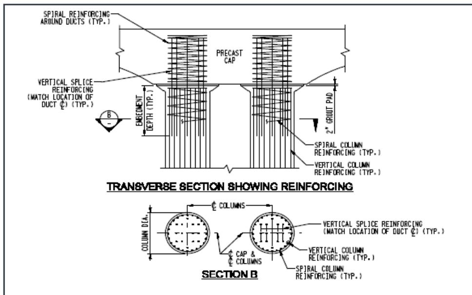
Figure 2.7 Precast column to precast pier cap connection
