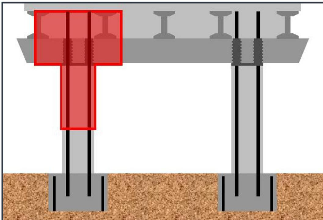
Figure 2.37 Column-cap beam connection with large diameter concept
