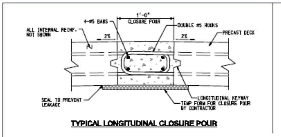
Figure 2.3 Full-depth precast concrete deck panel longitudinal connection
