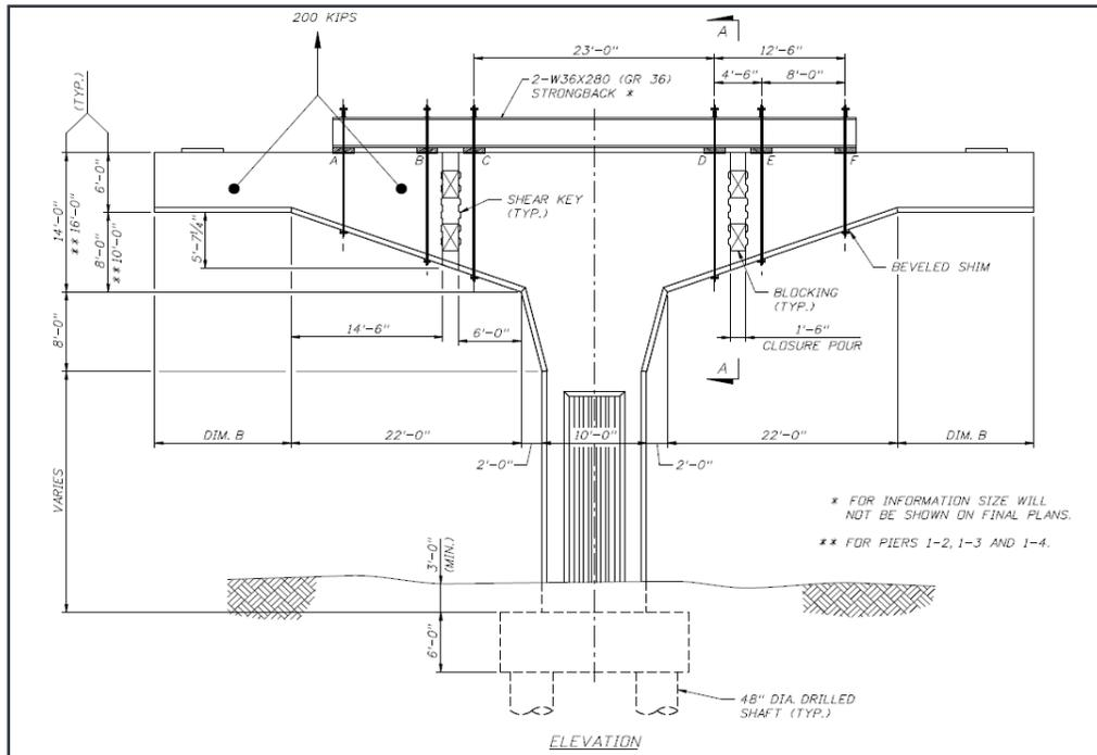
Figure 2.29 Segmental cap beam/pier system in Florida
