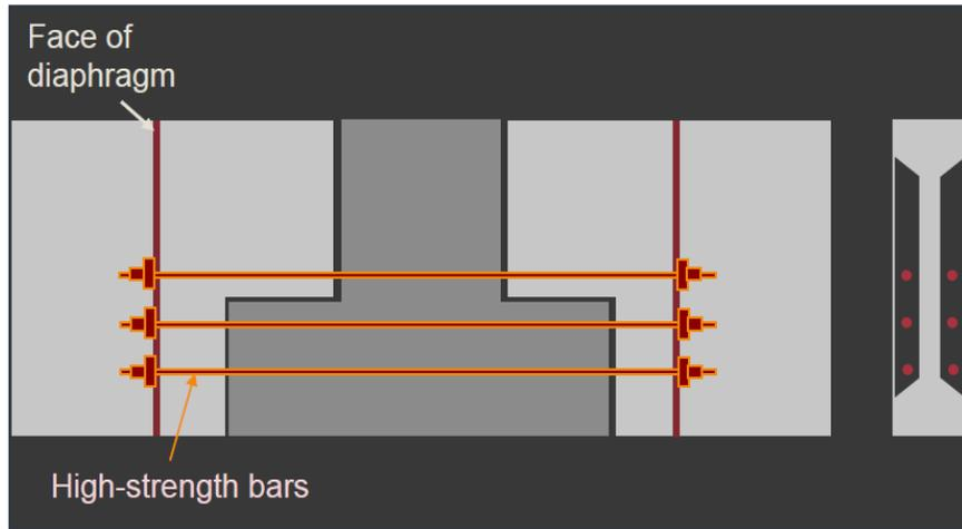
Figure 2.43 ISU superstructure/cap beam connection with high-strength bars
