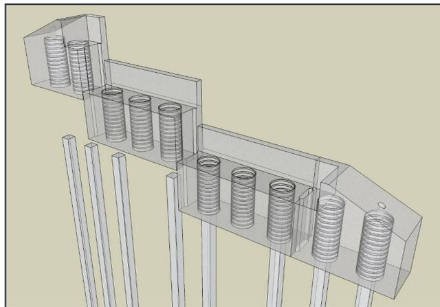
Figure 2.27 Precast abutment wall segments with embedded corrugated pipes<sup>56</sup>
