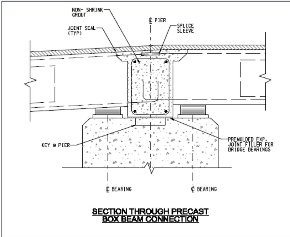
Figure 2.4 Precast box beam connection over pier cap
