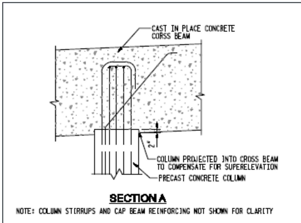
Figure 2.5 Precast column to cast-in-place cap beam connection
