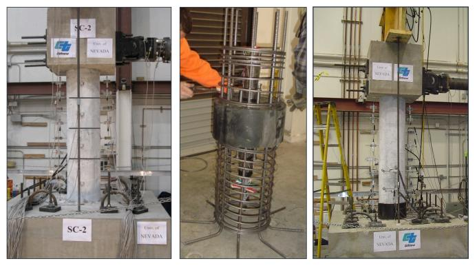
Figure 2.45 Segmental column model with CIP base segment on a shake table at UNR
