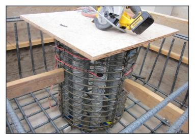
Figure 2.25 UNR test model with corrugated ducts in footing
