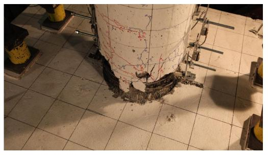
Figure 2.35 Plastic hinge in precast column embedded in CIP footing
