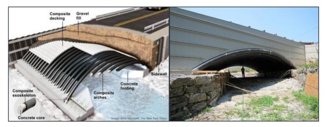
Figure 2.52 Concrete-filled carbon-fiber-reinforced polymer tube arches implemented in a bridge in Massachusetts
