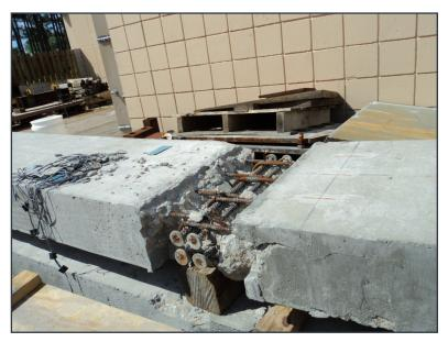
Figure 2.33 Full-depth deck slab connection model tested at the FDOT Testing Structure Research Center
