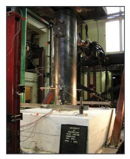
Figure 2.49 Concrete-filled steel tube column model tested at the University of Washington
