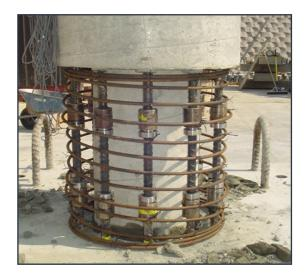
Figure 2.39 Precast column-footing connection model with headed bar couplers tested at UNR
