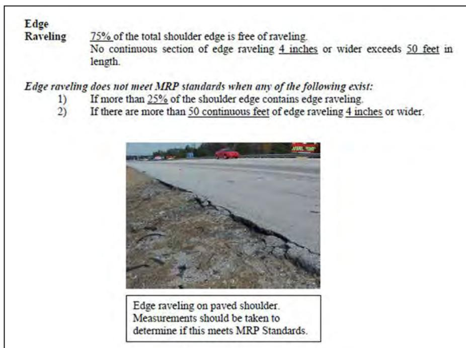
Figure 2.2 Example of a pass/fail rating criteria (source: FDOT)
