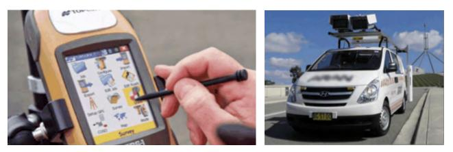
Figure 2.7A Handheld data-collection equipment
