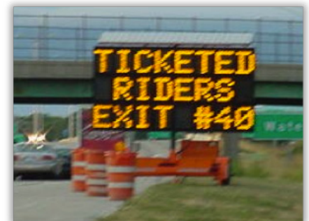
Figure 3.10 Temporary variable message signs are strategically placed to direct specific riders to the correct exit
