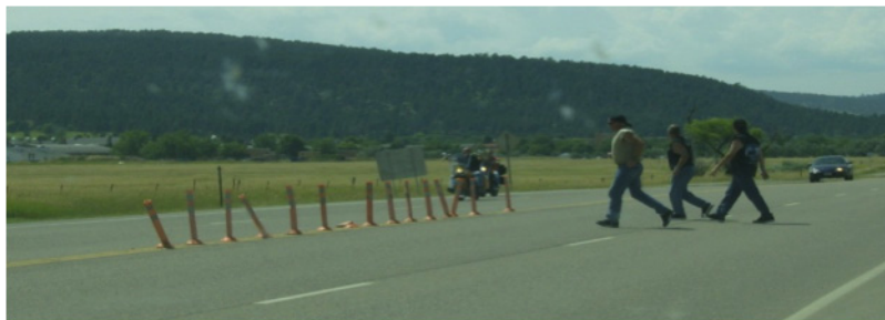
Figure 3.5 Temporary “candlestick” entrance control and lane delineation for a Sturgis motorcycle venue (photo courtesy of Doug Kinniburgh)
