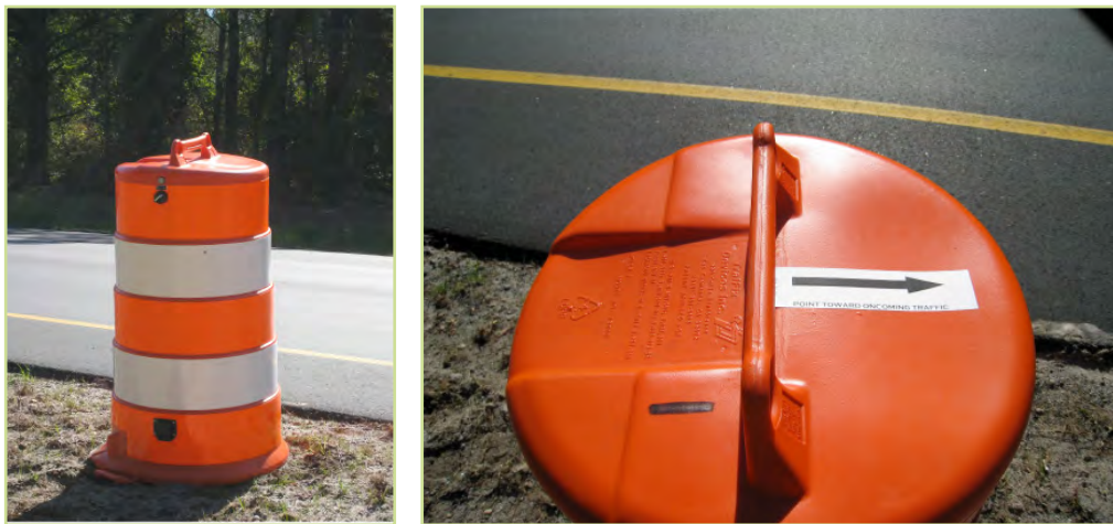
Figure 3.13 Portable work zone traffic data collection and communication technology
