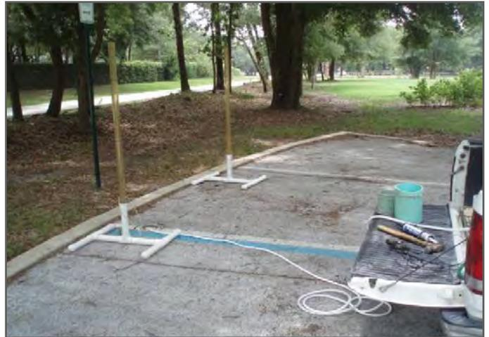
**Figure 4.16** Device developed at UCF for measuring infiltration of permeable pavements
