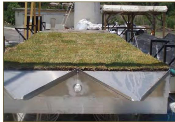
**Figure 4.22** Test bed for fertilizer wash-off study
