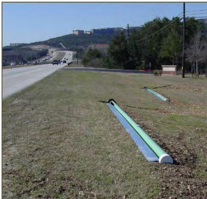
***Figure 4.10 Sample test setup of highway vegetated strips***
