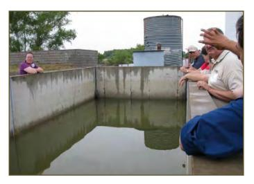
Figure 4.14 Nonproprietary stormwater vault prototype at TTI
