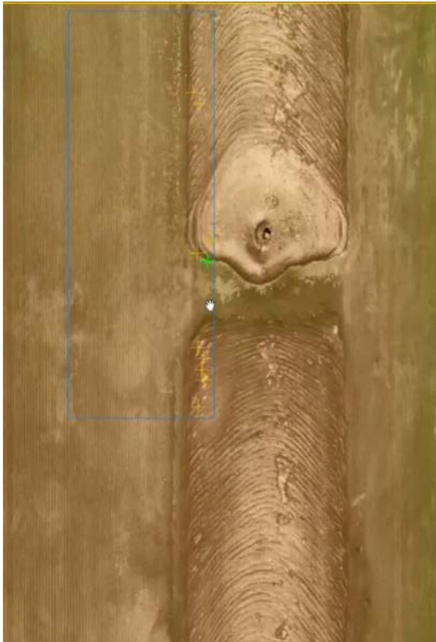
Figure 11. Point-cloud image of a weld scanned and rendered using KEYENCE equipment (Source: KEYENCE Corporation of America)
