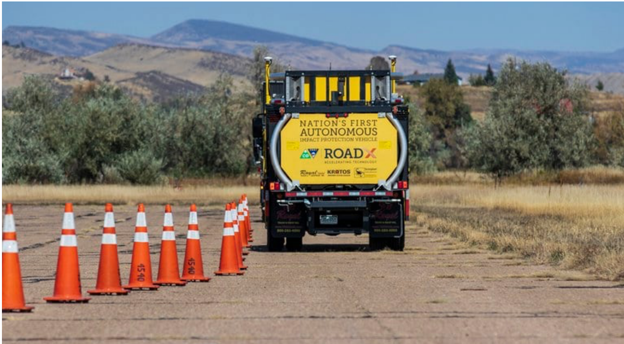
Figure 3: Colorado Autonomous Truck Mounted Attenuator (Source: Colorado DOT)
