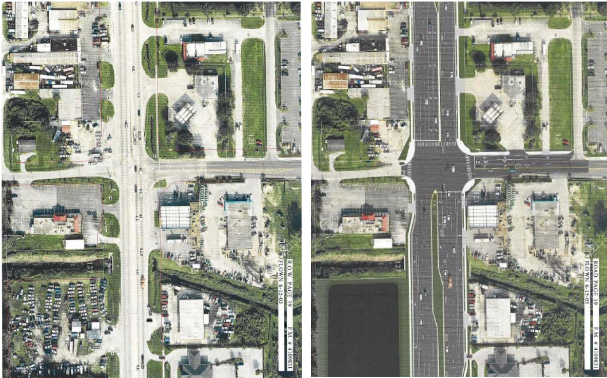
The two exhibits above illustrate ROW limits along SR 50, the first showing the limits of the state ROW (red lines) and the second exhibit showing the proposed reconstruction superimposed on the map. These mapping aids are of great benefit in illustrating for property owners the configuration of the planned construction.
