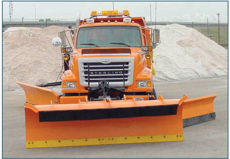
Figure 2-13. Snowplow truck with reversible plow and both right- and left-hand wings (UDOT)
