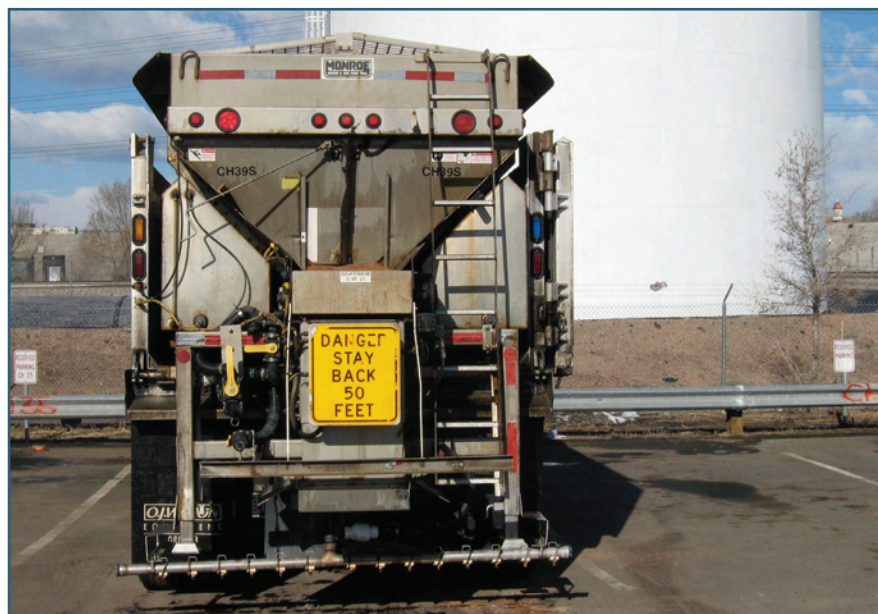
Figure 2-21. Saddle tanks tucked between the dump box and the V-box spreader carry liquid chemicals for prewetting solids. (City/County of Denver, CO)
