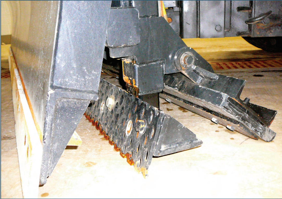
Figure 2-19. Triple-blade experimental plow with steel carbide (cutting), serrated (scarifying), and rubber (squeegee) blade (INDOT)
