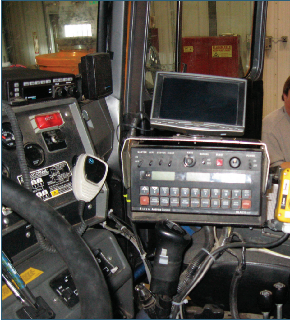
Figure 1-3. The modern snowplow truck is crammed with screens, keyboards, toggle switches, and other controls. (CDOT)
