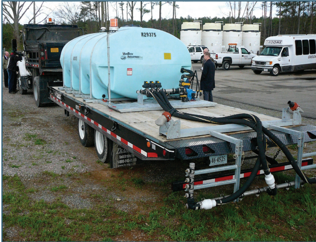
Figure 2-27. Flatbed-mounted 3,000-gallon liquid chemical spreader (VDOT)
