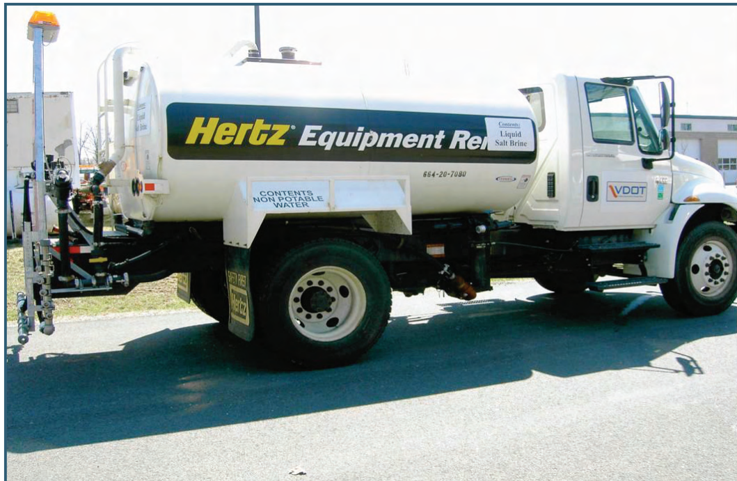
Figure 2-28. Water truck available for off-season rental to spread liquid chemicals (VDOT)
