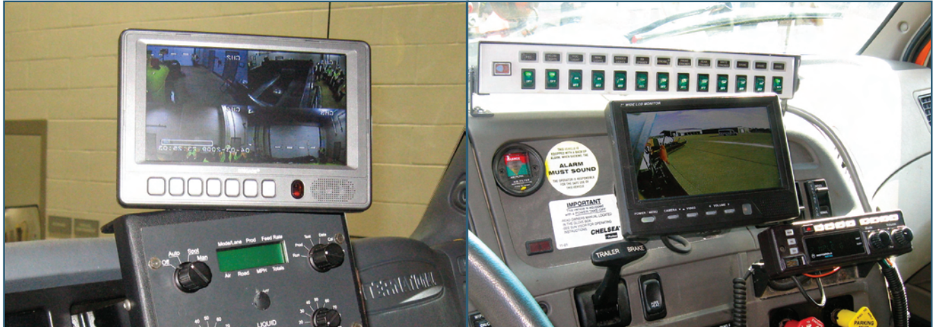
Figure 2-30. Video camera views are displayed in the cab so that the operator can know what is going on to the right, left, rear, and front of the truck, including in the spreader box (left). A tow-plow behind the truck (right). (INDOT, Mn/DOT)
