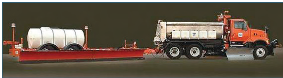
Figure 2-14. Tow-plow equipped with liquid spreader (Mn/DOT)
