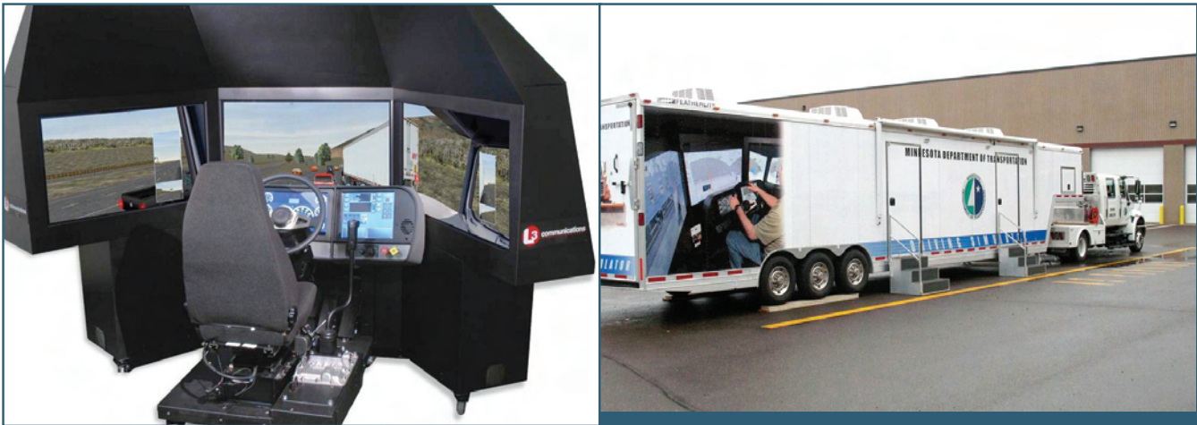
Figure 2-45. Training simulators are becoming popular for training snowplow operators, especially when the workforce has high turnover or is drawn from flexible or cross-trained staff. (Mn/DOT)
