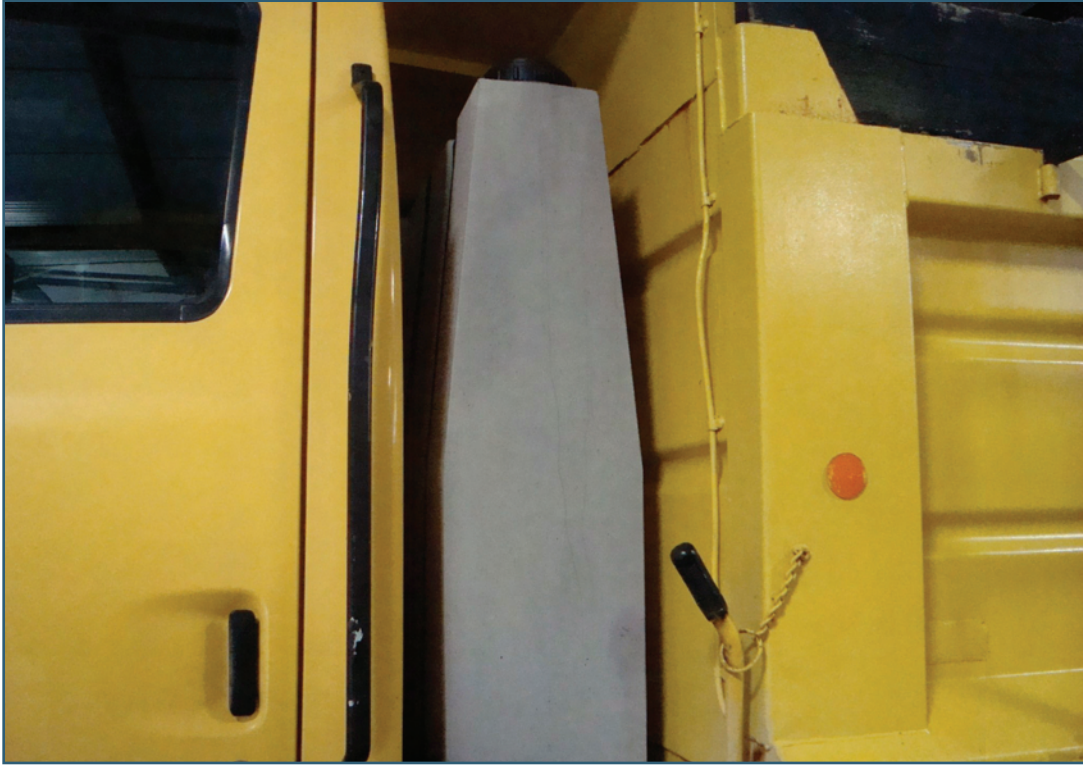
Figure 2-22. Liquid chemical storage between the cab and box (INDOT)
