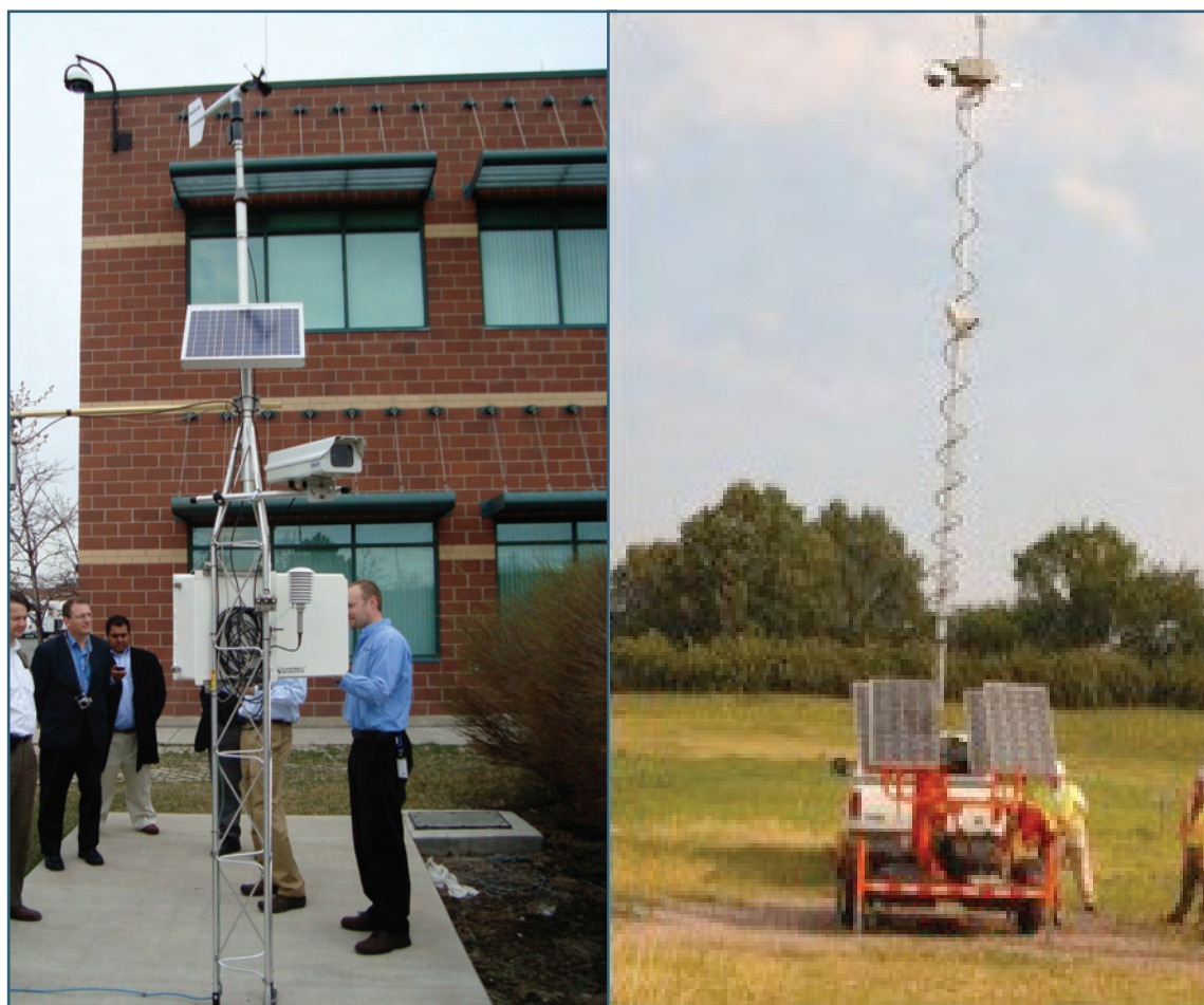
Figure 2-34. These low-cost, portable RWIS data-gathering stations are solar-powered and camera-equipped. (UDOT, VDOT)
