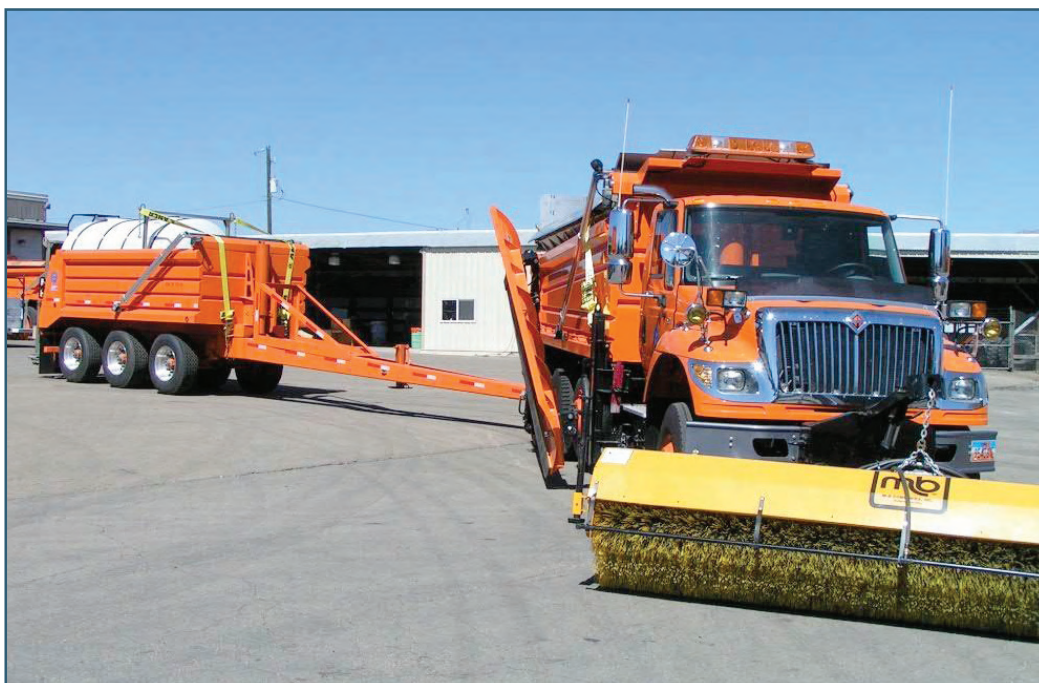
Figure 2-16. Rotary-power front-mounted brooms for removing lightweight snow (Note that this unit also uses a tri-axle pup trailer to spread liquid chemicals.) (UDOT).
