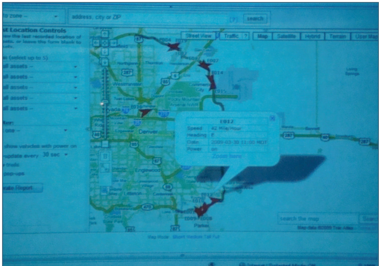
Figure 2-6. The dispatcher is able to monitor the location, speed, and direction of the plow trucks. (E-470 PHA)
