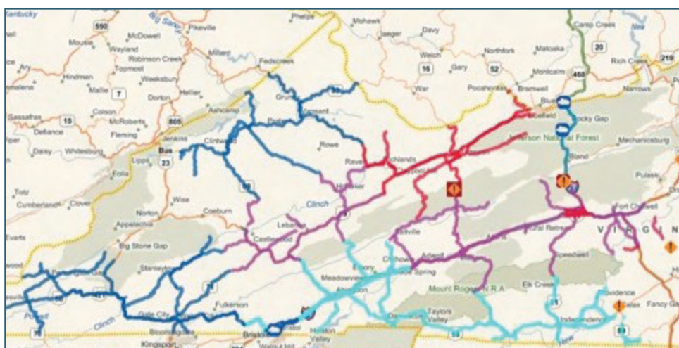
Figure 2-10. The higher frequency of AVL readings can produce accomplishment graphics showing routes completed.
