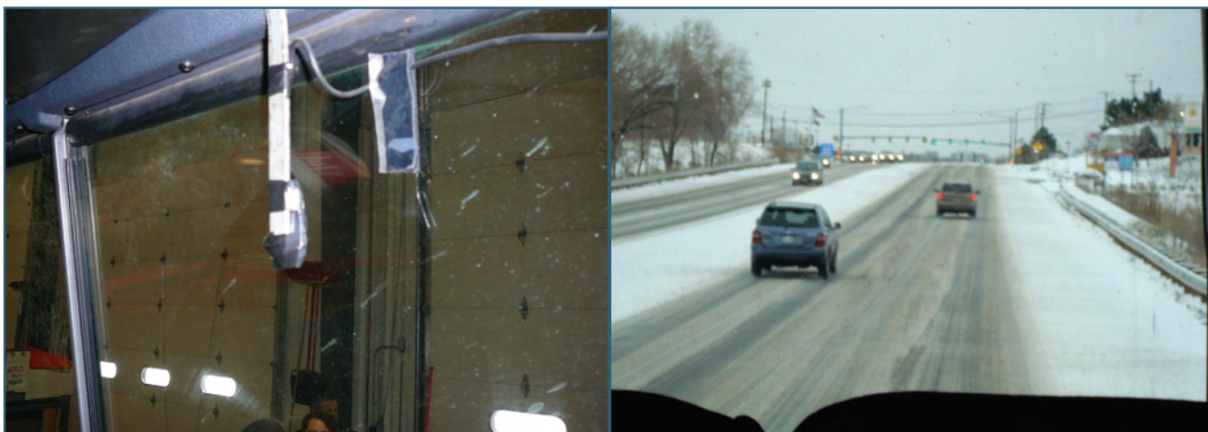
Figure 2-29. In-cab video camera mounted on the passenger side of the windshield is capable of sending to the dispatcher pictures of the road and weather conditions as they actually exist from the driver's view (CDOT)
