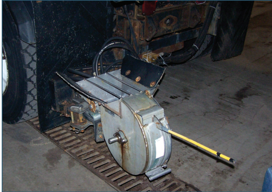
Figure 2-23. The latest zero-velocity chemical spreader being tested by Mn/DOT is designed to discharge chemicals straight back at zero velocity with respect to the ground. (Mn/DOT)
