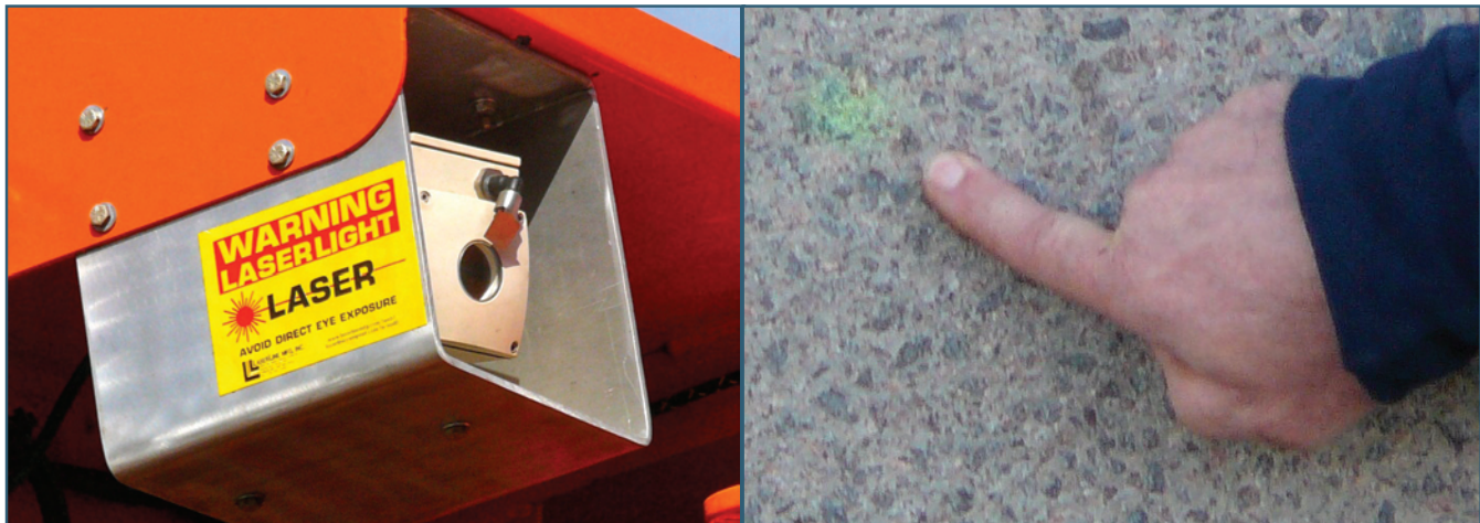
Figure 2-32. A laser beam system projects green light onto roadside snow to show the operator how far out the wing or tow-plow extends. (Mn/DOT)
