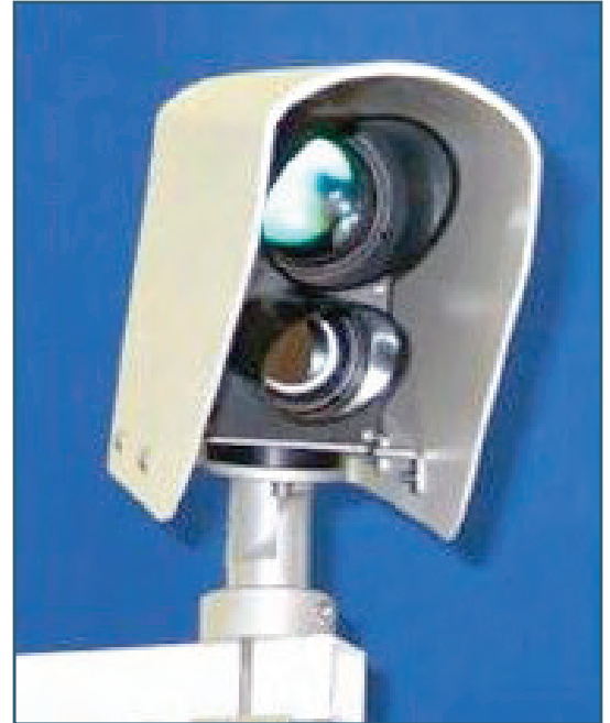
Figure 2-35. Noninvasive surface sensor identifies the presence of water, ice, slush, snow, and frost and provides an indication of slipperiness. Unlike pucks, which are embedded in the pavement, these sensors are mounted alongside or above the road.
