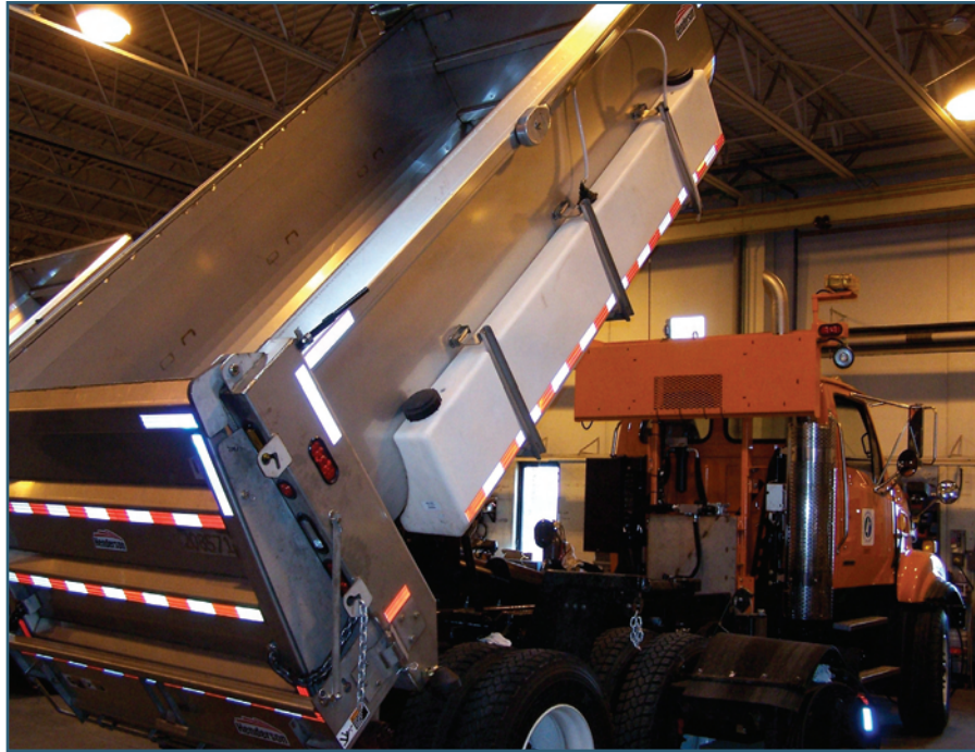
Figure 2-20. Saddle tanks on the side of the dump box carry liquid chemicals for prewetting solids and are used in conjunction with tailgate sanders for solid chemicals. (Mn/DOT)
