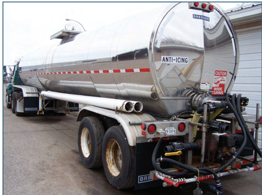
Figure 2-26. Typical 5,000-gallon trailer-tanker for spreading liquid anti-icing chemical and resupplying storage tanks at local garages (Mn/DOT)
