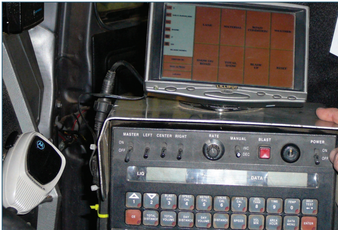
Figure 2-3. Operators can choose from a menu within reach while they are operating the vehicle. (INDOT)
