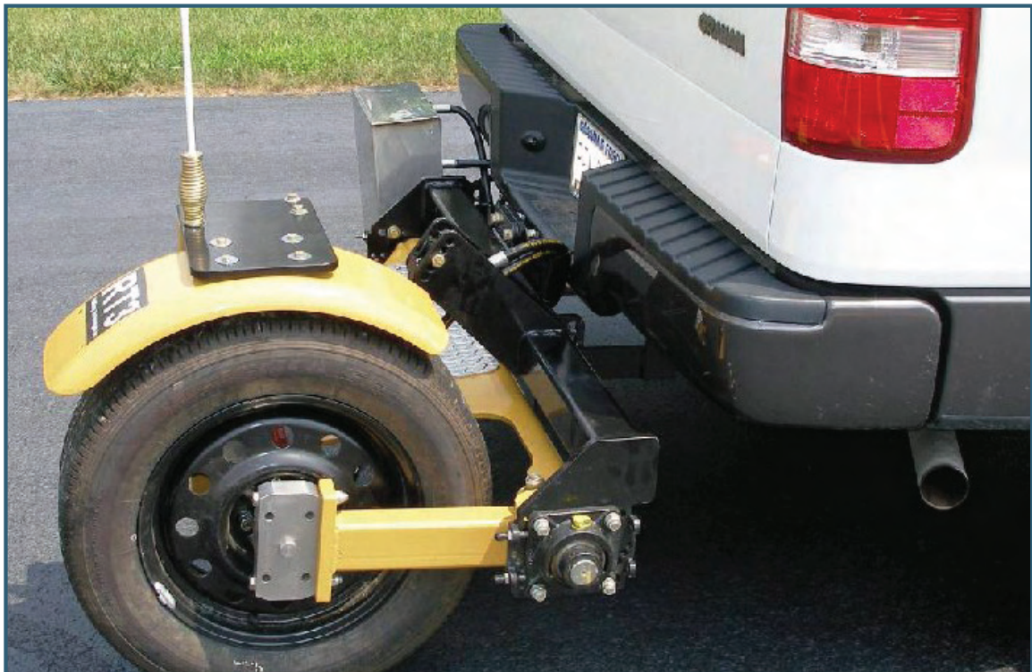
Figure 2-36. Friction measurement device being experimented with in Utah. (UDOT)
