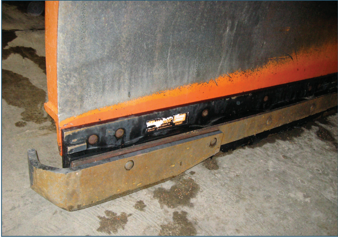
Figure 2-17. Rubber blade reinforced with front steel blade and steel curb protection (CDOT)
